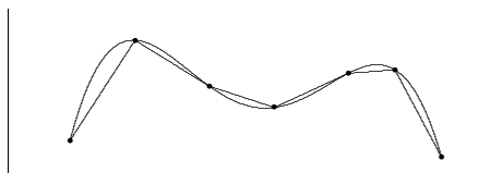
Figure 11.8 Approximating arc length with line segments.
