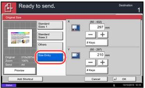
When you have selected [Size Entry], press [+] or [-] to set the sizes of *X* (horizontal) and *Y* (vertical). By pressing [# Keys], you can use the numeric keys.
