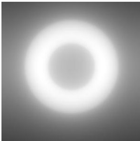
FIGURE 10. The reconstruction of the function E using unfiltered backprojection. Image created using MATLAB.
