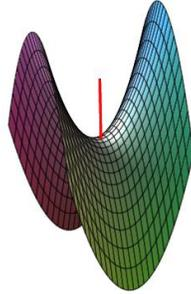
Figure 22: A point (indicated by the red line) with negative Gauss curvature
