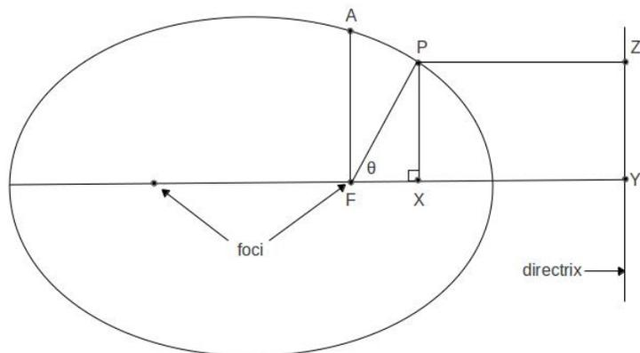
Figure 3: Important points in a conic section
