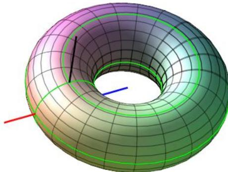
Figure 23: Torus containing points with all three curvature types (red = elliptic, black = parabolic, blue = hyperbolic)
