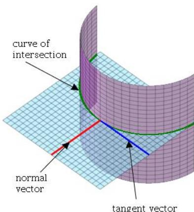
Figure 19: Finding the normal curvature of a point on a cylinder
