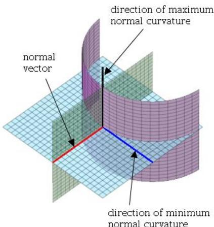
Figure 20: Finding the principle curvatures of a point on the cylinder in equation (43)
