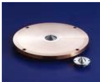
Figure 5.2. Photograph of a Sampler (the larger one) and a Skimmer Cone for ICP-MS.
