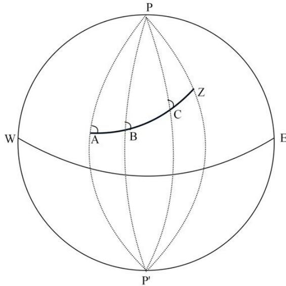
Figure 3: Rhumb line path intersecting meridians at same angle [3].
