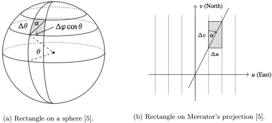
Figure 8: Transformation from spherical to rectangular coordinates.
