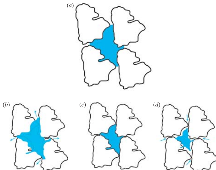
Fig. 2. Schematic showing three possible responses of solvent to cooling. (a) The room-temperature crystal, with the portion in blue illustrating the solvent occupying the interstitial space between the four macromolecules in the unit cell. (b)–(d) The crystal with its low-temperature packing arrangement, and three possibilities for solvent contraction. (b) The solvent shrinks less than the interstices, resulting in the extrusion of solvent into the neighboring interstices. (c) The solvent shrinks by the same amount as the interstitial space. Some solvent rearrangement is required to accommodate the lattice repacking. (d) The solvent shrinks more than the interstices, resulting in import of solvent into the interstice from neighboring ones.
