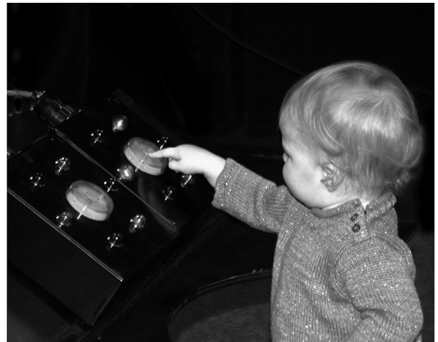
Figure 1. The boxes and the experiment setup. Two custom-designed boxes, each with a large central button and surrounding colored lights. The correct target is cued by a flashing light under the large central button. When the cued button is pressed, surrounding lights flash and an interesting sound emits from the box.
