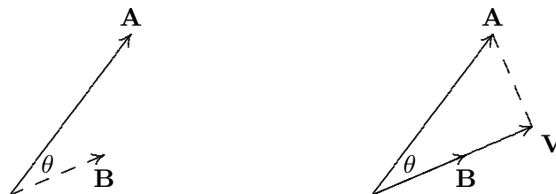
Figure 14.7 \mathbf{V} is the projection of \mathbf{A} onto \mathbf{B} .
