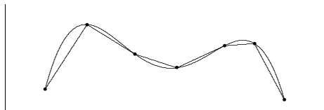
Figure 11.4.2 Approximating arc length with line segments.
