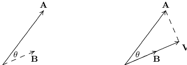
Figure 12.3.4 \mathbf{V} is the projection of \mathbf{A} onto \mathbf{B} .
